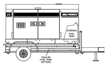
Figure 32. Internal Fuel Tank System
